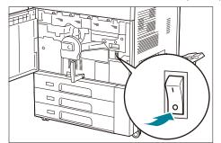
The Power/Power Saving indicator goes out on the control panel.
