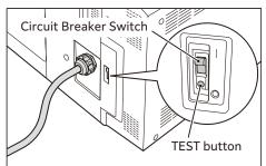
**3.** Check that the switch is turned off and in the "O" state.
