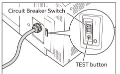
When fault current is detected, the circuit breaker is automatically turned off to discontinue the electrical flow. Do not touch the breakers under normal condition. For information on fault current, refer to the "Safety Notes".
